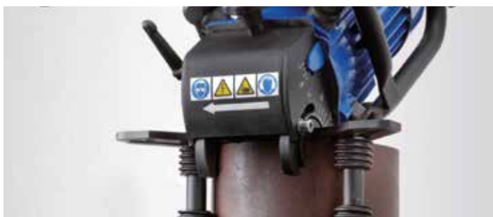
Edge processing of pipes in vertical position.
