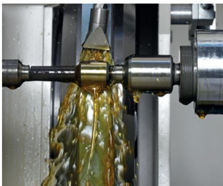
Sharpening BDS core drills
