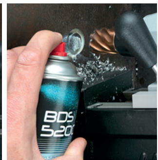
Step 2: During drilling, spray high-performance lubrication spray onto the tip of the drill and into the borehole.
